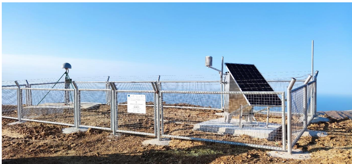
31 July 2021 – ALEV00CYP GNSS CORS Station at Alevga Site
